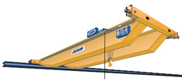
The measurements A1, C1 and K1 can be changed by adjusting to existing build conditions, by pushing up the bottom of the main girder up to the bottom of the end carriage.
